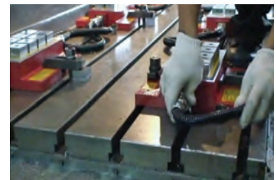
Connect the control cables to chucks and control
