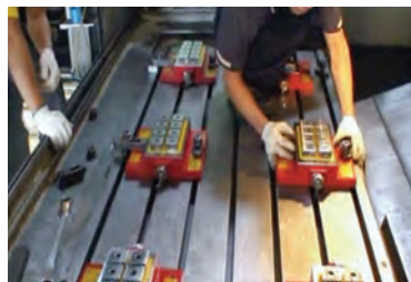
Position the chucks on the machine bed
