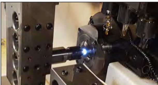
Guide bushing camera, aligning ID tool
