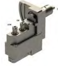
B07-GSA-207-2X Angled Drilling / Milling Arbor Size: ER11 Output: 1:1 Adjustable 90° Internal Coolant-Thru Machine: B01/02/07
