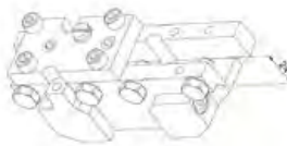
DE20-OF-020 Tool Holder Tool Size: 16x16mm Height 24mm
