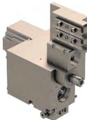
P03-GSC-117-S Main Block Tool Holder Collet Size: ER11 Output: 1:2 Tool N°01 cutter carrier 8mm x 8mm Tool N°02 cutter carrier 8mm x 8mm Tool N°03 high frequency \varnothing 25 Tool N°04 in ER11 with RPM 16'000. Tool N°05 is a modular quick change for different operation. Machine: P034H
