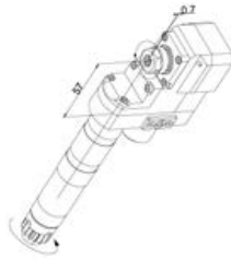
GSE-708 End Drill/Mill Collet Size: ER11 Output: 1.65:1
