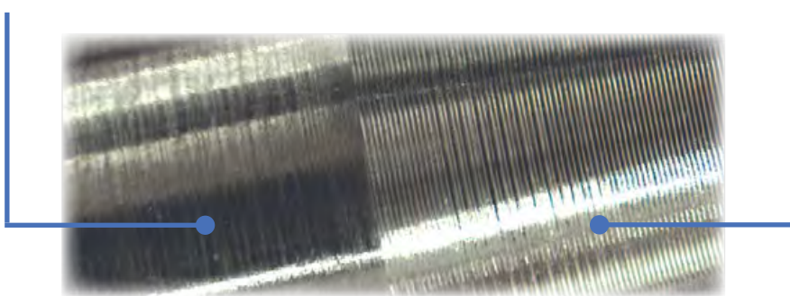
Turned With A multidec® TOP Wiper Insert
