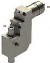
B026-RSE-110-IK Axial Drilling / Milling Collet Size: ER16 Output: 1:1 Internal Coolant-Thru Double-Ended Machine: B026/32/38
