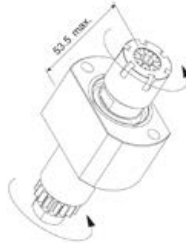
E20-GSE-110 End Drill/Mill Collet Size: ER16 Output: 1:1
