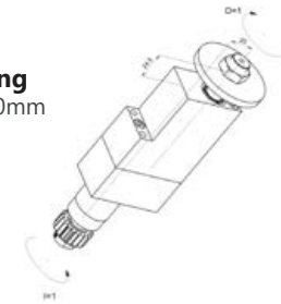
GSC-1307-DEC Slitting Saw Arbor Size: Ø16mm Output: 1:1 Max Tool Ø: 63mm Max Tool Width: 6mm A 2 20VII
