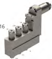
SR32J-GSE-3710 End Drill/Mill Collet Size: ER11 ER16 Output: 1:1 Double Ended
