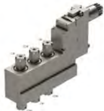
GSC-1310-HP Cross Drill/Mill Collet Size: ER16 Output: 1:1 High Pressure Coolant G1/8 Fitting [PN#4005-000104]
