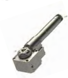
LSW-101-L20 Thread Whirling Ring: Utilis Output: 1:1 3,9, or 12 insert cutter, Adjustable ±10°
