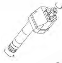
GSE-316-GS End Drill/Mill Collet Size: ER16 Output: 1:1
